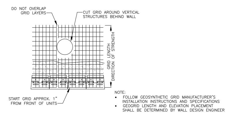
GEOSYNTHETIC AT STRUCTURES BEHIND WALL
